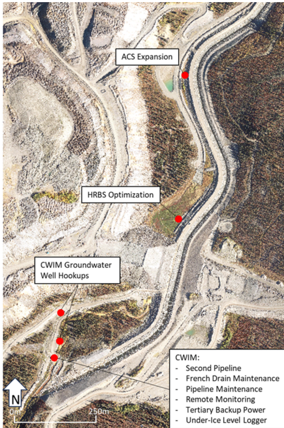
Map of planned upgrades to improve contaminated water capture in the NFRC area (November 2024).
