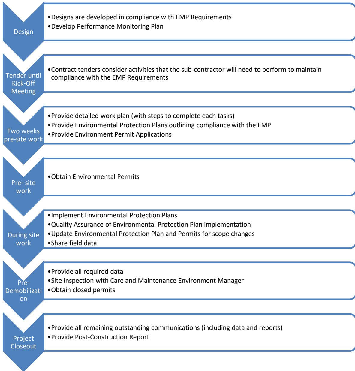
Figure 2: Work Package Alignment with the EMP
